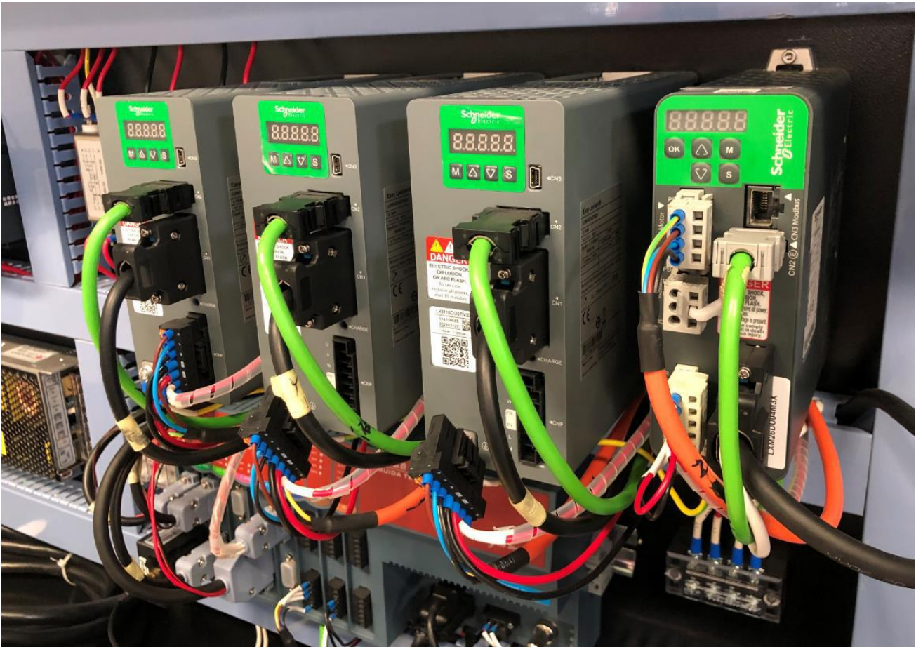
Schneider servo motors and drivers. Motor reducer is SHIMPO.
