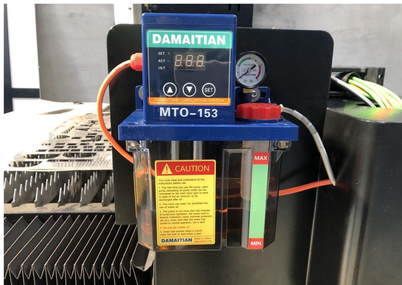
It automatically lubricates guide rails, which ensures the machine keep moving smoothly and with good precision.
